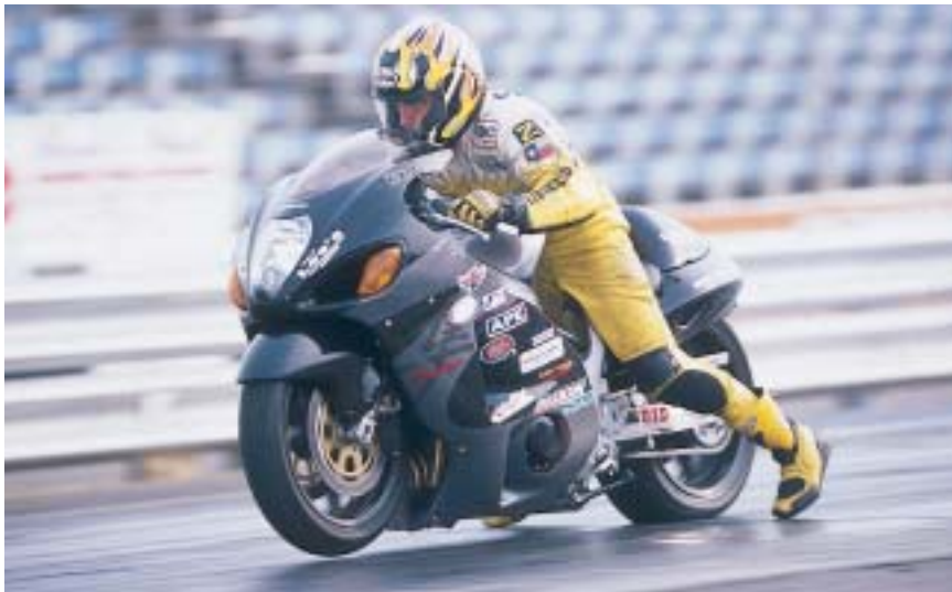
Shierts' drag Hayabusa launches ferociously off the line. With 370 horsepower and over 170 ft./lbs. of torque feeding through a lockup clutch, I was hoping to let this bike get me into the 8.5-second bracket (which Shierts has done easily). I'll be back for another shot at it.
