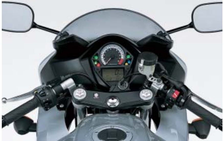
The SV650's gauge package is shared with the 1000, as are the new push-to-pass and hazard light switches.
