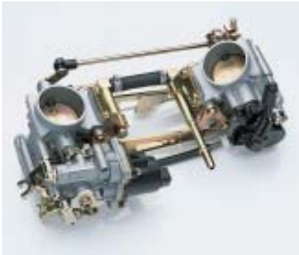
The old SV's carburetors are replaced with Suzuki's SDTV injection setup with 39mm throttle bodies, which—like the GSX-Rs and SV1000—incorporate secondary throttle valves controlled electronically.
