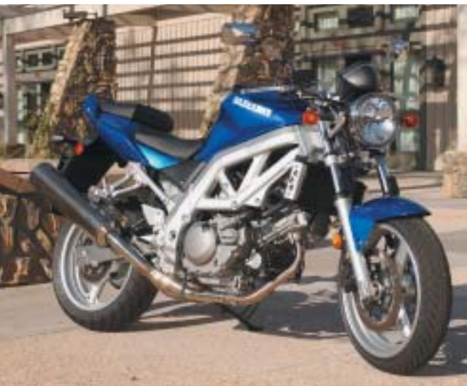
In addition to the obvious differences between the S and non-S models, the unfaired SV has a slightly longer swingarm and wheelbase, footpegs that are lower and further forward, one-tooth-shorter final gearing and a hair more trail thanks to triple clamps with 1.5mm less offset. Note the new oil cooler on both versions.
